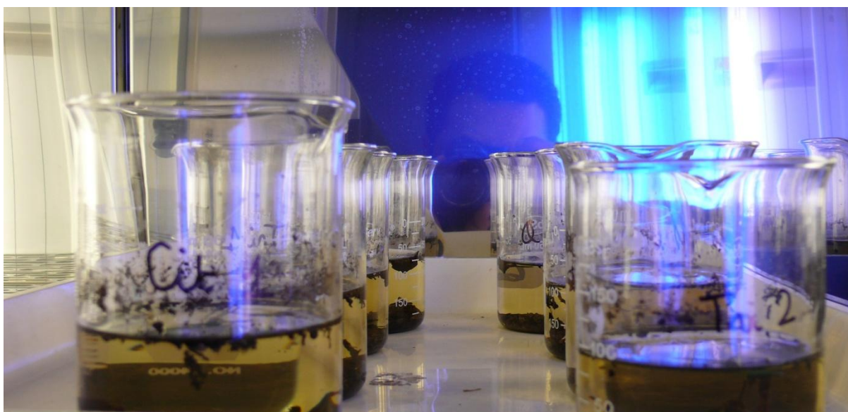
Plate 4: Leaf-bait soil bioassays after 4 days incubation in blue and cool white fluorescent light
