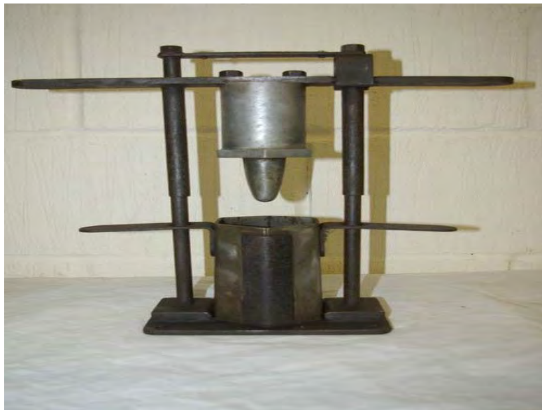
Figure 90. A Gorodam soil block-making machine as used at Waipoua Nursery.
