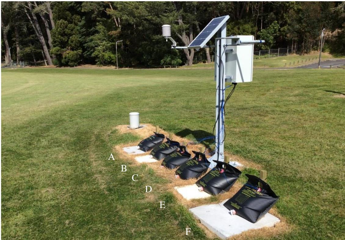
Figure 1: Weather station and monitoring of temperature potential of solar radiation for degradation of *Phytophthora* taxon *Agathis* oospores. Bags A and F were maintained on cement slabs, B and E on polystyrene boards and C and D were kept on the ground. The temperature within each bag, ambient temperature, solar radiation and relative humidity data were captured hourly using a Campbell CR1000 data logger.
